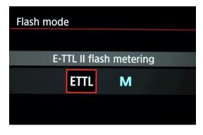
During the initial tests, dependently of concrete camera, strobes condition, batteries etc., photographer should set small constant (+/-) correction to TTL Flash exposure control. Pay attention on this.
