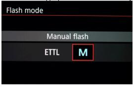
In such Manual mode also becomes available flash output level scale in submenu. User can adjust flash output level by camera wheel, looking to this menu scale (or looking to camera service screen):
