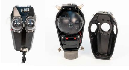
mechanical switch-on button with double o-ring and a little window in At the base of the housing there are 10 plexiglass which allows to visualise the internal camera display.
